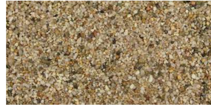
Paving Type 3: Resin-bound gravel surface to bitmac along the promenade (width to match existing adjacent Cardiff Pointe) and to the path through Public Open Space. PCC flat-topped edge restraints to path through POS. 150 x 225 decorative concrete up stand kerb to Promenade
