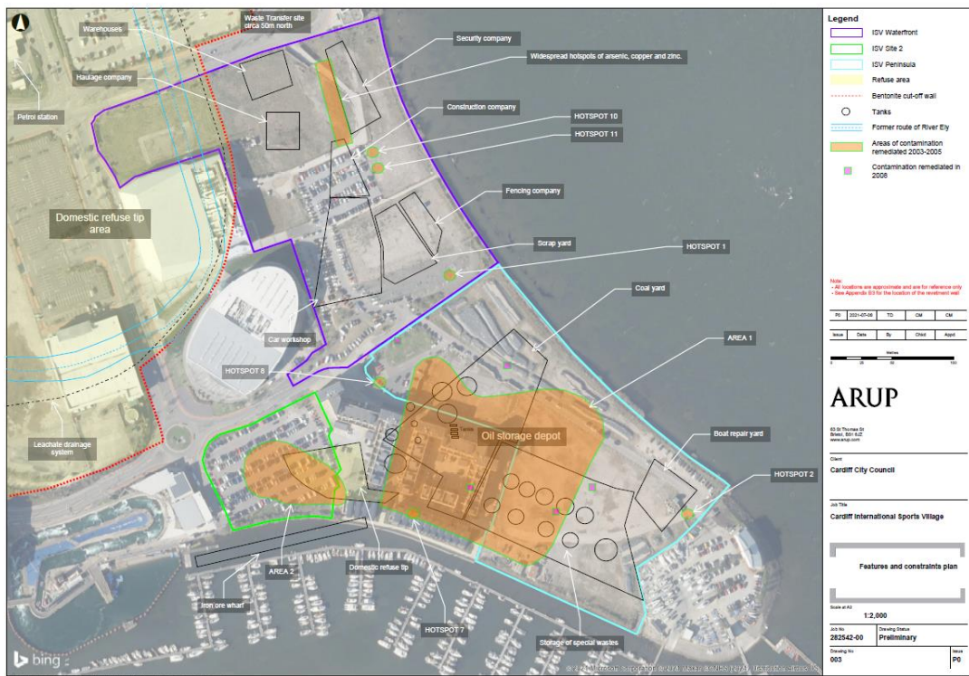
Figure 5.4 Areas Subject to Remediation in 2003-05 (Source: Drawing 003 from Arup Technical Due Diligence Note, Dated 2021 (Ref: 282542-00))
